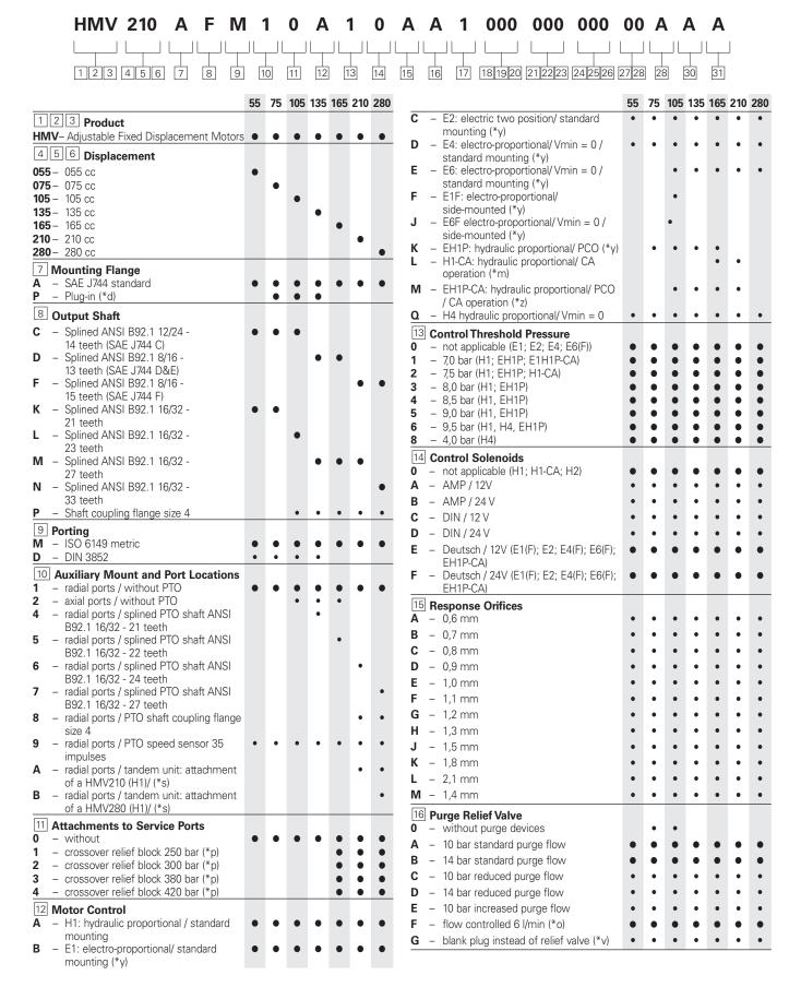
**HMV Variable Displacement Motors** (Open & Closed Loop Operation)
