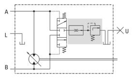
Flow-controlled purge flushing in an open loop circuit approx. 4 I/min at 5 bar set pressure (independent of low pressure) diagram 4
