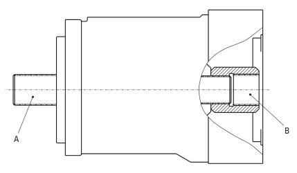
The diagram Torque transmission of HMF / A / V / R shows the output side (A) and the PTO throughshaft (B) of a motor.
