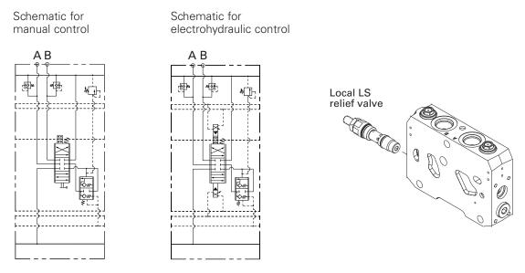
Note: Post Comp Section Load Sense relief prohibits flow share if multiple sections containing local load sense reliefs are operated simultaneously. Available with LH build only
