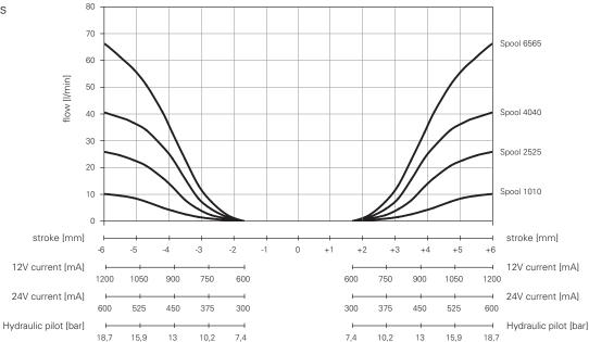
14 bar  $\Delta$ p between load sense and inlet pressure
