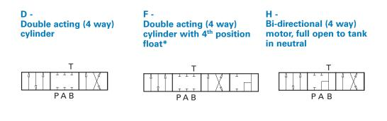
Note: Spool F requires additional valve body machining and special 4th position detent selection
