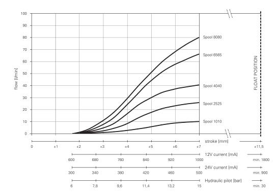
Typical work port auxiliary valve curves
