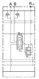
Schematic for electrohydraulic control
